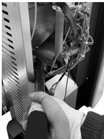
Fig. 106 - Reiniging omgevingsventilator (Atena³ Plus 12/14 - Duke 12/14 At - Saba 12/14)
